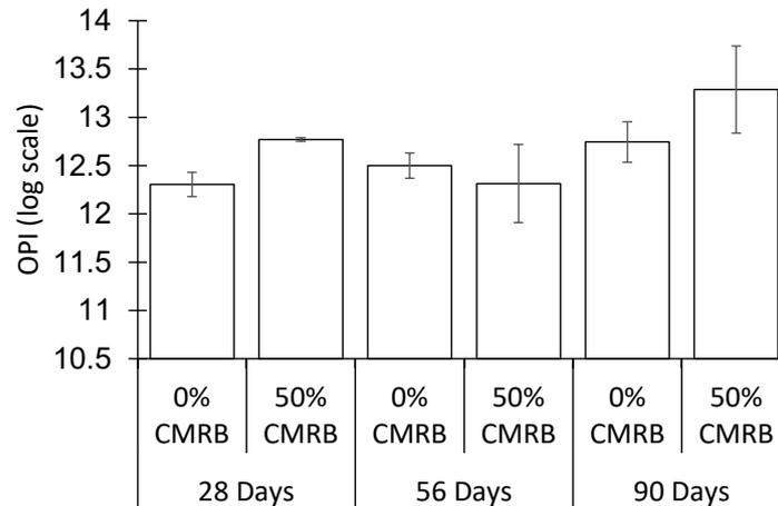
Figure 4: OPI for concrete made using 0 and 50 % CMRB as fine aggregates at 28, 56 and 90 days.
