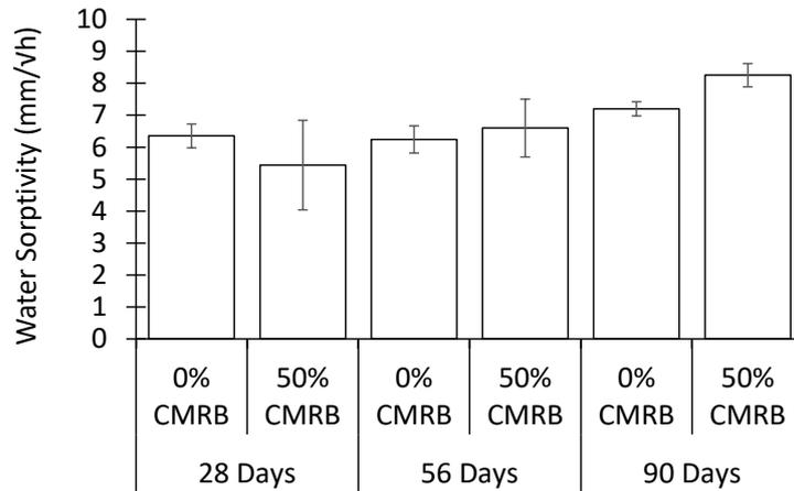
**Figure 5: Water sorptivity for concrete made using 0 and 50 % CMRB as fine aggregates at 28, 56 and 90 days.**
