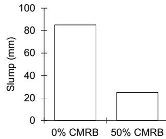
**Figure 2: Slump results for concrete made using 0, 50% CMRB as fine aggregate.**
