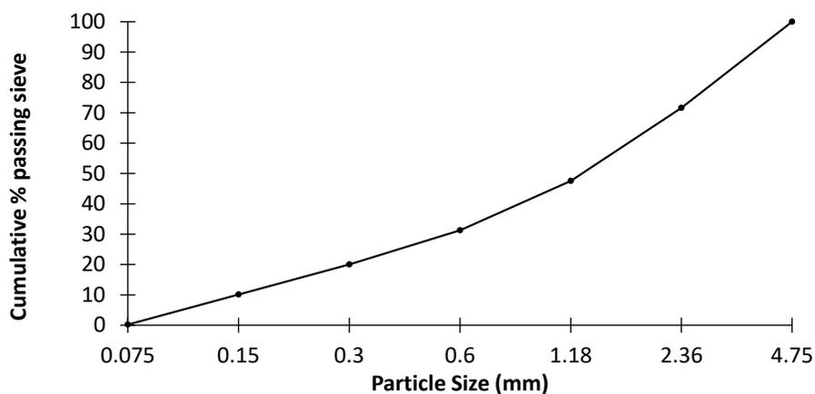
Figure 1: Grading profile for natural fine Andesite aggregate
